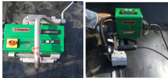
Picture 8 : welding machine for fusion welding
